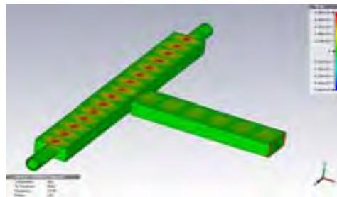
In another simulation, a water drop is placed inside the cavity at a fixed position (at a maximum of the E-field). When plotted with a cut along the x axis through the half x-dimension of the rectangular cavity (Figure 4), it is possible to observe how the drop disturbs the E-field while absorbing the microwave energy, thus increases its temperature. A virtual sphere and planes are drawn surrounding and splitting the drop for a better appreciation of its interaction with the field.
